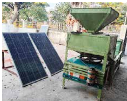
Solar operated charoli decorticating machine
