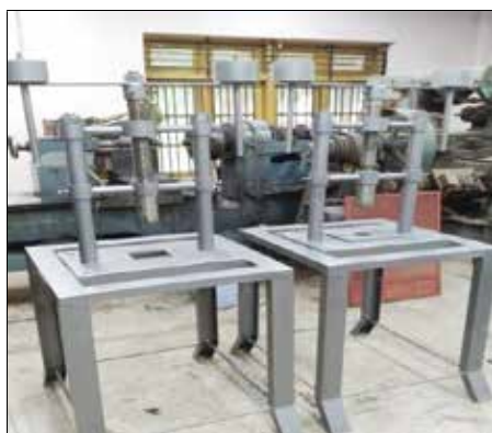
Wax Thread Extruder Machine for Dhokra Craft
