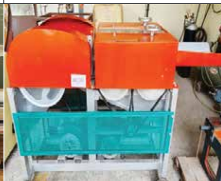
Bamboo Chipper Machine
