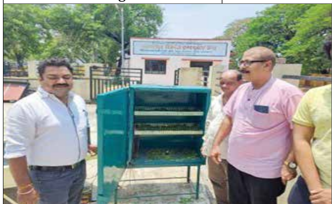
Solar operated charoli decorticating machine
