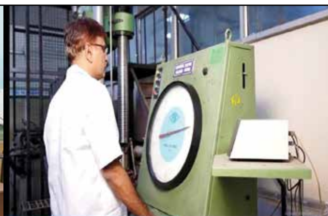
UNIVERSAL TENSILE TESTING 1000KN AT MSME-TS HYDERABAD
