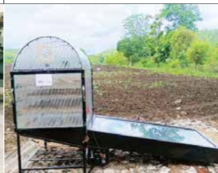
Combo Solar dryer (Air forced & tunnel Dryer)
